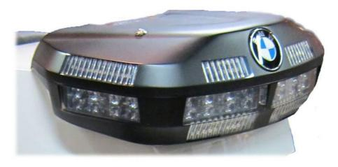
• Rear and rear-side facing emergency lights provide greater intensity than the previous double-stacked units.
